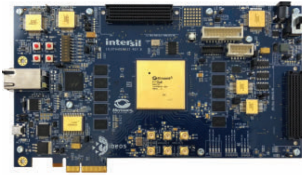
Renesas Electronics Corp. has created a radiation-hardened version of the Microsemi RTG4 field-programmable gate array (FPGA).
