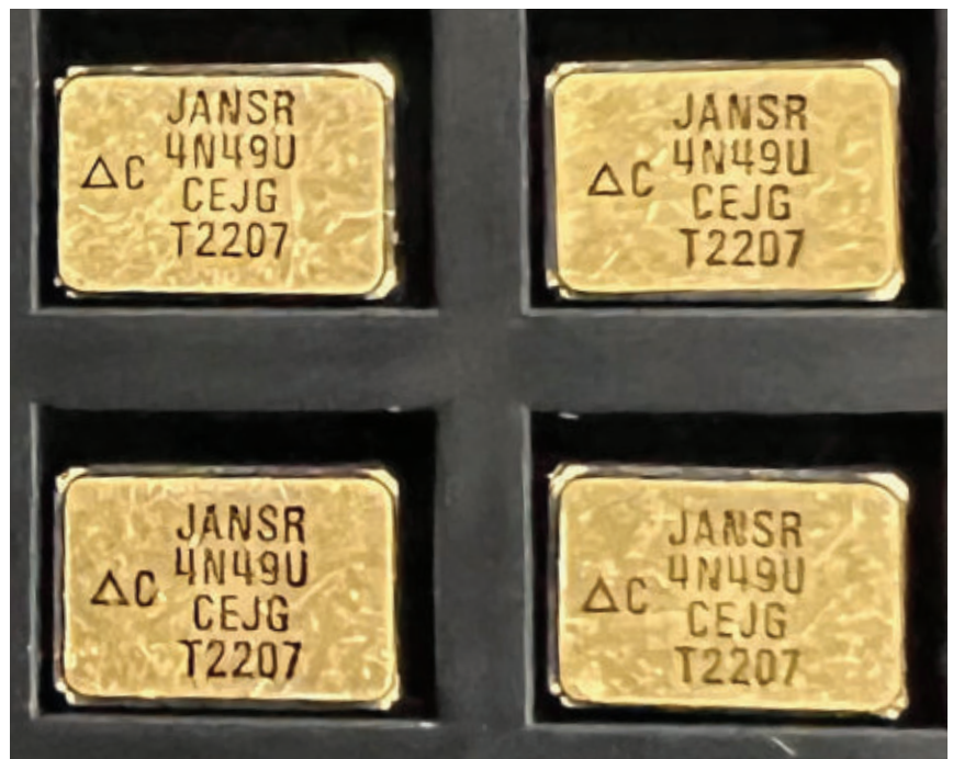
Micropac Industries specializes in radiation-tolerant optocouplers that help isolated circuits communicate with one another. Pictured is the Micropac JANSR 4N49U
