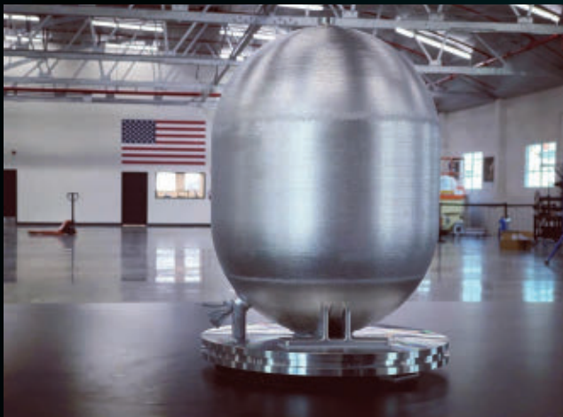
Velo 3D collaborated with Launcher on orbiter propellant tanks.
