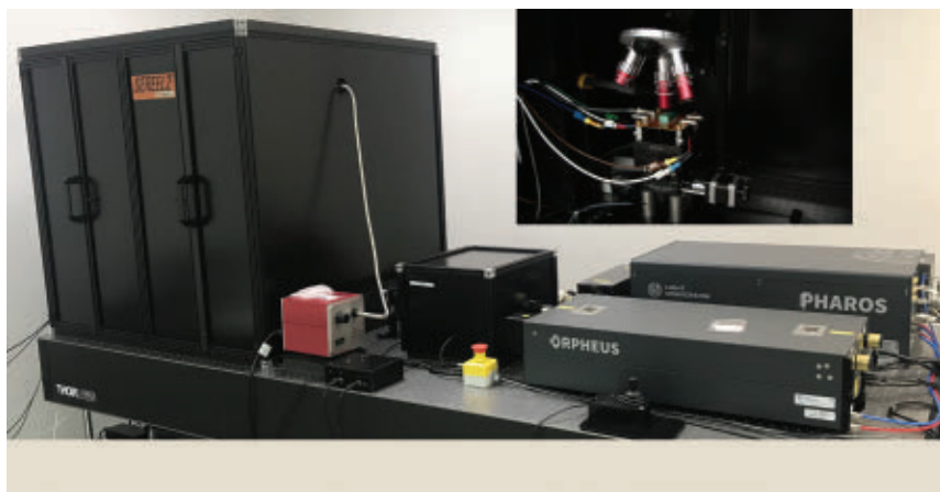
Radiation testing is crucial for finding electronic parts that can survive in space. Pictured is the Radiation Test Solutions SEREEL2 test system for single-event upsets.
